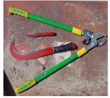
FIG. 17 THORN REMOVAL KNIVES AND PRUNER
