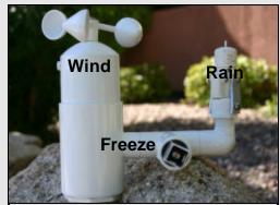
Irrigation shutoff devices. Clockwise, from upper left: rain, wind and temperature.
