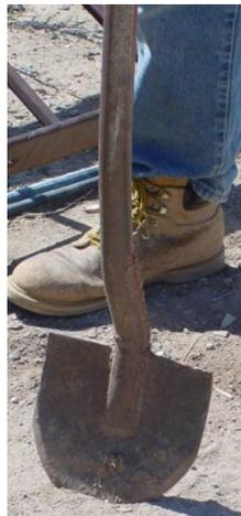
**FIG. 33 MODIFIED SHOVEL FOR OFFSHOOT REMOVAL**
