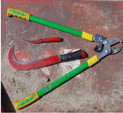
**FIG. 17 THORN REMOVAL KNIVES AND PRUNER**
