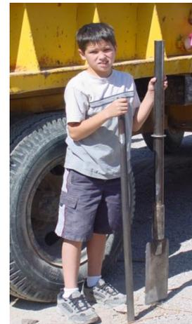
**FIG. 34 CHISEL AND SLAMMER**
